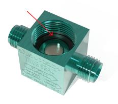
**7.** With Valve domes facing upward, place the two Valve Diaphragms above the Sealing Washer, making sure the diaphragms are placed in the same order they came out.
