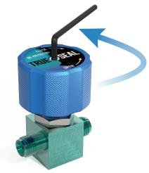
2. Be sure to have the valve in the open position and loosen the Actuator Stem Guide with a 1/2" socket and a standard wrench with a 9-10" handle in the Counterclockwise direction. Then separate the Actuator Stem Guide from the Valve Body.
