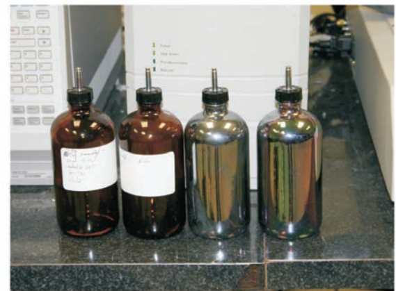
Figure 3 - Amber and Silonite Coated Bottle-Vac Glass Canisters used for Sulfur Stability Study
