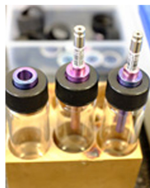
Fig. 1 Sorbent pens and vial closures used for extraction of phenols by VASE
