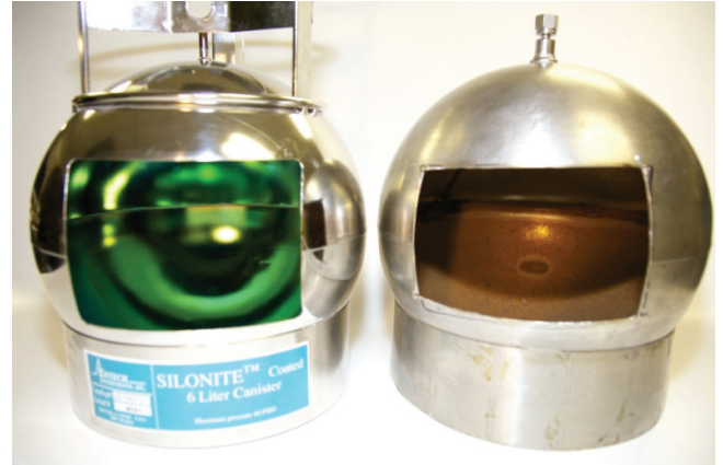
Figure 1 - Canister on the left is silica coated, whereas the rusty canister on the right is uncoated stainless steel, which is more subject to corrosion without the protective ceramic layer.
