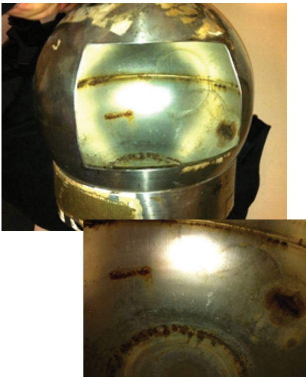
Figure 4 - A canister which looks good on the outside can have rust and weld scars on the inside that will affect the stability of TO15 compounds.
