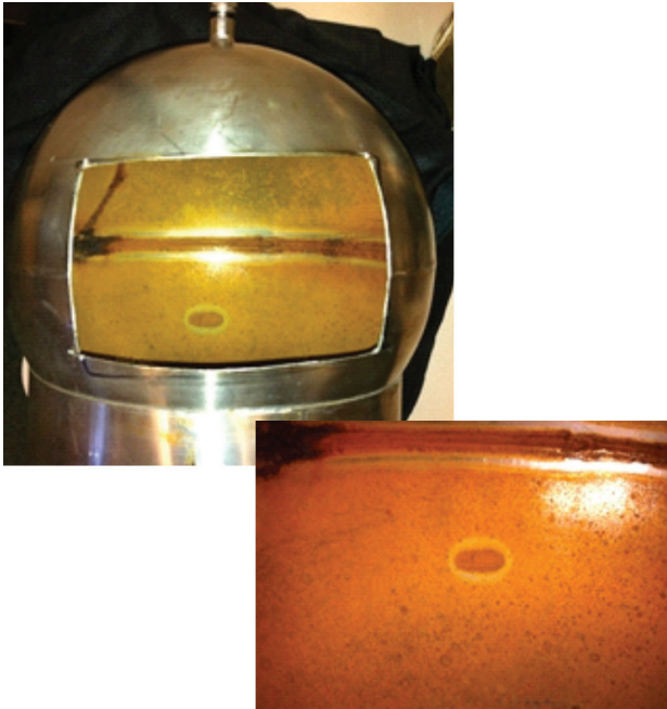
Figure 3 - This rusty canister was still in use by a laboratory until it developed a leak.
