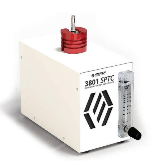
Figure 3 - A 3801 Sorbent Pen Conditioner (Entech Instruments) was used to initially condition the Sorbent Pens. During the analysis, the Sorbent Pens are desorbed to the GCMS and thoroughly baked out, eliminating the need for additional thermal conditioning before reuse.
