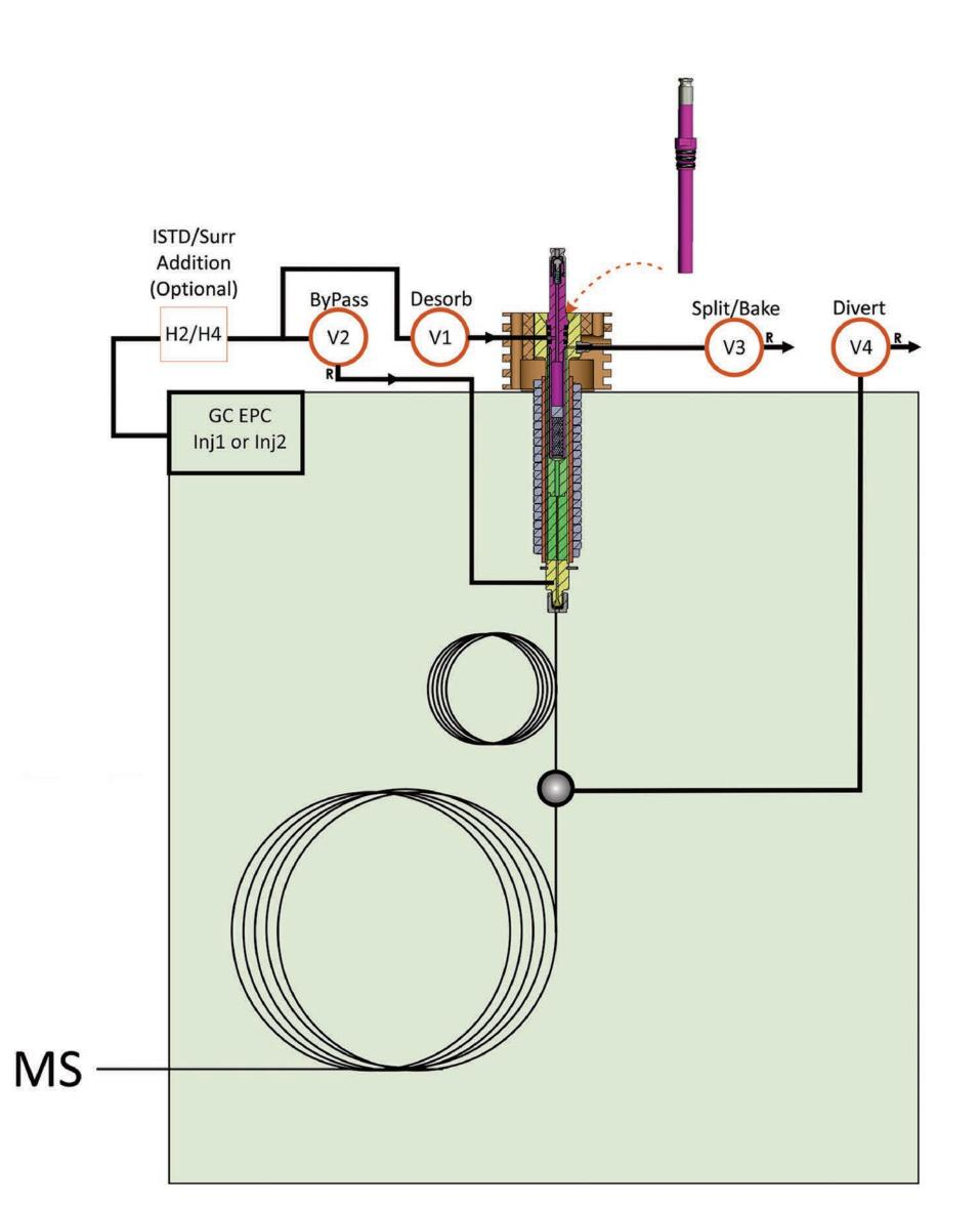
**Figure 5** - The 5800 installs into an available GC injection port position, providing gas flow control through 4 separate valves. Dairy samples in this study were analyzed both splitless at 6:1, and by using a large volume splitless technique where the V3 split valve remains off, while the V4 valve turns on to allow faster desorption and splitless pre-loading of heavier volatiles onto the pre-column.
