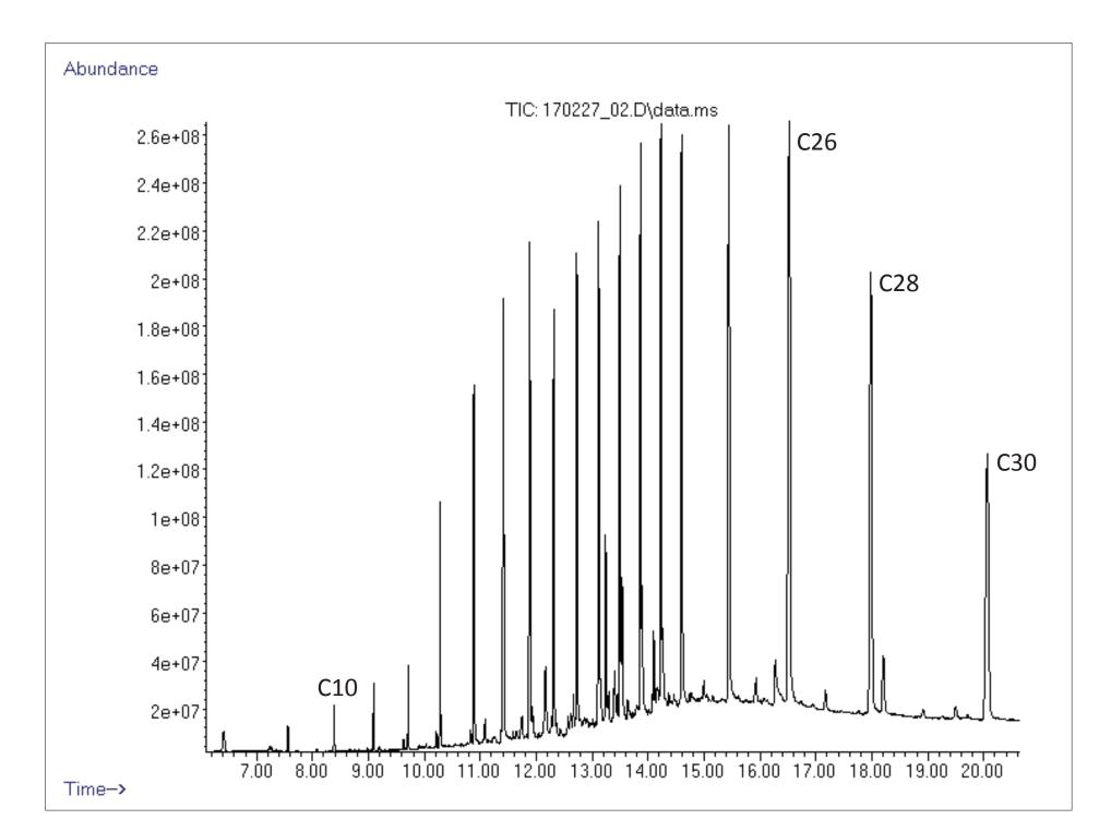
Figure 6 - C8 to C30 Calibration Standard, used to verify proper system operation, including recovery out to C30 prior to sample analysis.
