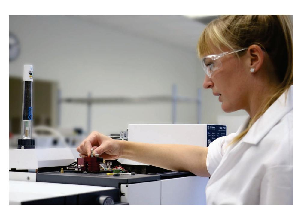
Figure 4 - The 5800 Sorbent Pen Desorption Unit (Entech Instruments) was installed on a 7890/5977A, allowing split or splitless desorption of the Sorbent Pens into the GCMS.
