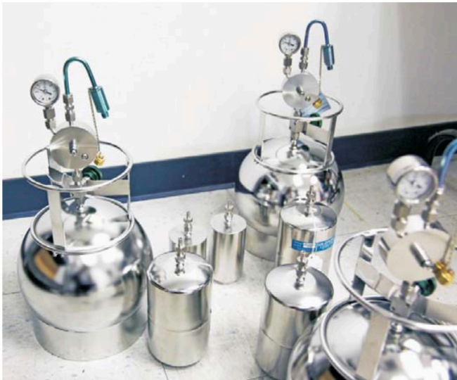
6L Classical Sampling canisters collecting 24 hour samples along side smaller 1.4L and 0.45L HDS samplers.
