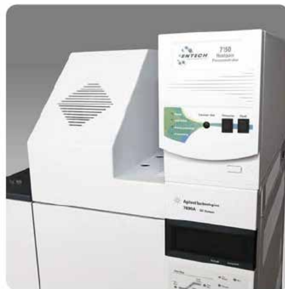
Figure 4 7150 Preconcentrator shown on an Agilent 7890/5975. The compact design was accomplished by using Dean's Switching rather than rotary valves for flow control. Separation of electronics and pneumatics modules allow the 3-stage trapping system to connect very close to the GC oven for improved SVOC recovery, while creating ideal modularity for an enhanced support strategy.
