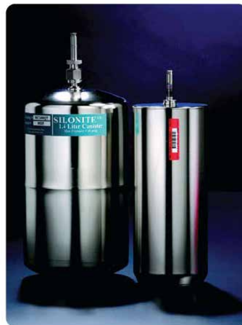
Figure 1 1.4L and 600cc Silonite™ coated MiniCan™ sampling canisters. MiniCans offer a no power, “pump free” sampling solution using an internal vacuum. The interior has a GC-like Silonite™ coating ideal for storing highly reactive compounds such as ammonia gas and phosphorous containing CWAs, allowing heating to as high as 150°C with very little increase in reactivity.
