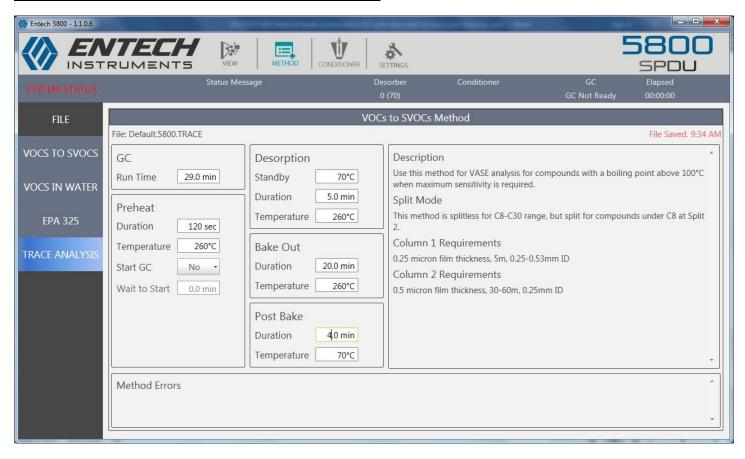
**Method Description:** Use this method for VASE analysis for compounds with a boiling point above 100°C when maximum sensitivity is required. A mass spectrometer is the recommended detector. Examples include ultra-trace level analysis, geosmin, 2-MIB, TCA, THC.
