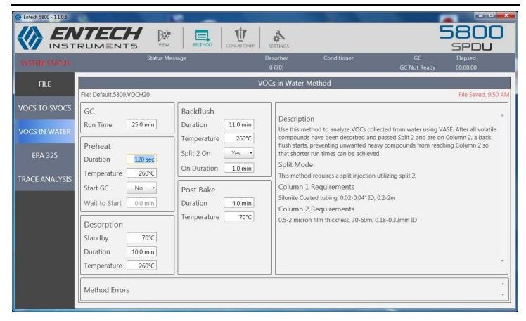
**Method Description:** Use this method to analyze VOCs collected from water using VASE. A mass spectrometer is the recommended detector.
