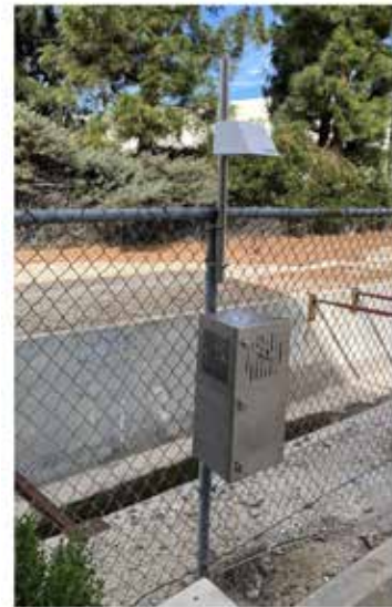
Figure 4 - Sample site B at Entech in Simi Valley, CA shown with a canister enclosure to support both sample collection techniques.
