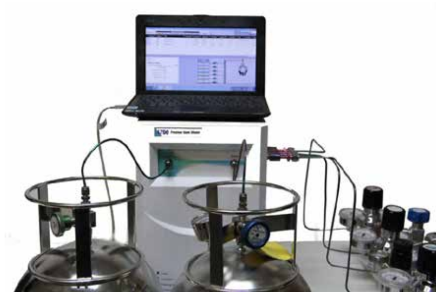
Figure 2 PPB Level Standard on left attached to input CH6 to create sub-PPB standard mixes into canister on the right. This approach is ideal for making low level calibration standards and for inertness testing field sampling canisters with a 1PPB mix.
