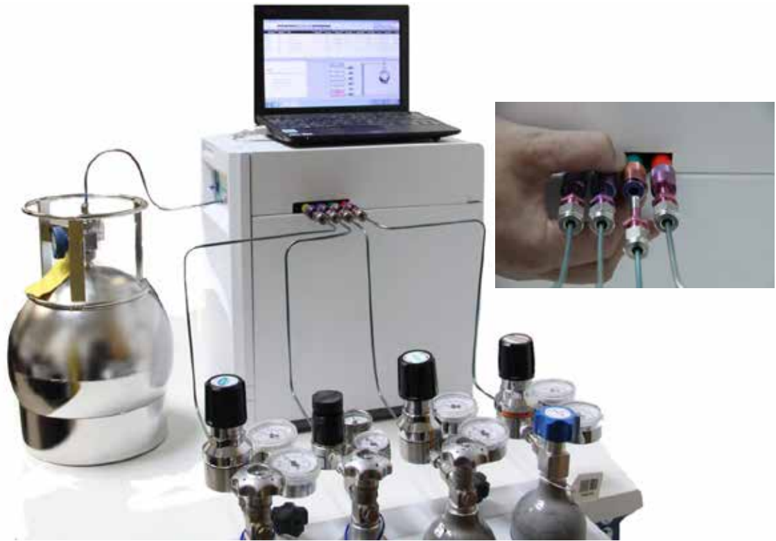
Figure 1 4700 with four 6R cylinders attached through side Micro QT Quick Connect Ports for rapid exchange of cylinder standards
