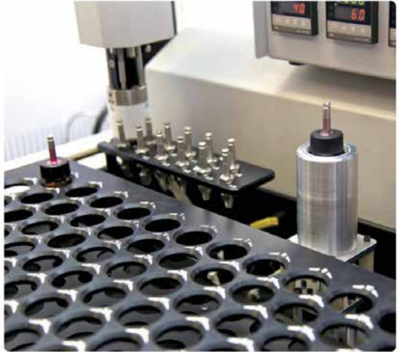
Figure 6 Entech Instruments, Inc. 7500A shown with mixing oven. Mixing oven facilitates rapid sample headspace equilibrium prior to the withdrawal of 10mL of headspace into the 7150 Preconcentrator.
