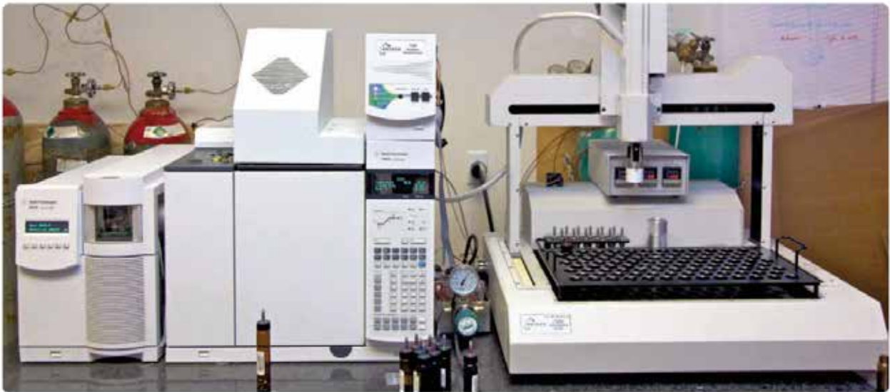
Figure 3 7150 / 7500A Automated 8260 Analysis System shown with Agilent 7890 / 5975 GCMS.
