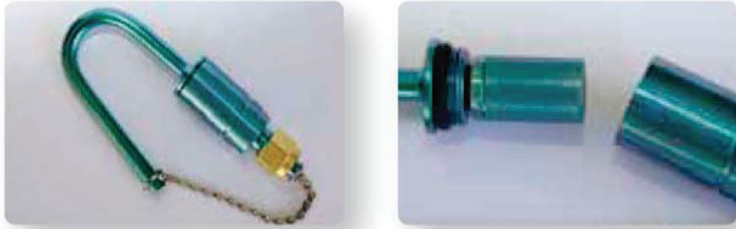
Figure 2 All inlets and inline filters are Silonite coated, as a standard feature, as non-coated filters and inlet lines were shown in the previous 902 application note to cause loss of heavier TO14 compounds. The need for extreme inertness has increased further with the inclusion of polar compounds in TO15, along with the requirements to drop detection limits well into the part-per-trillion range.
