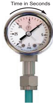
CS1200Ex + 6L Canister - Time to drop from 20" to 10" Hg
