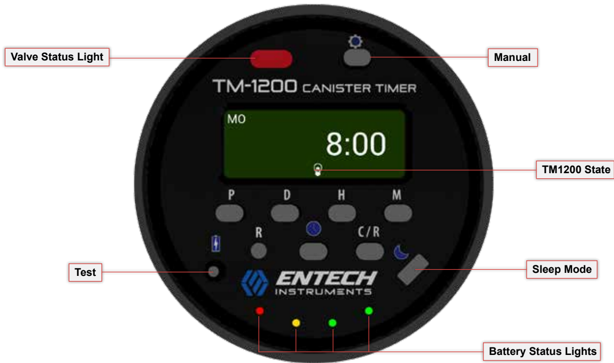
Figure 1.3 - TM1200 Lights, Controls, and Statuses.
