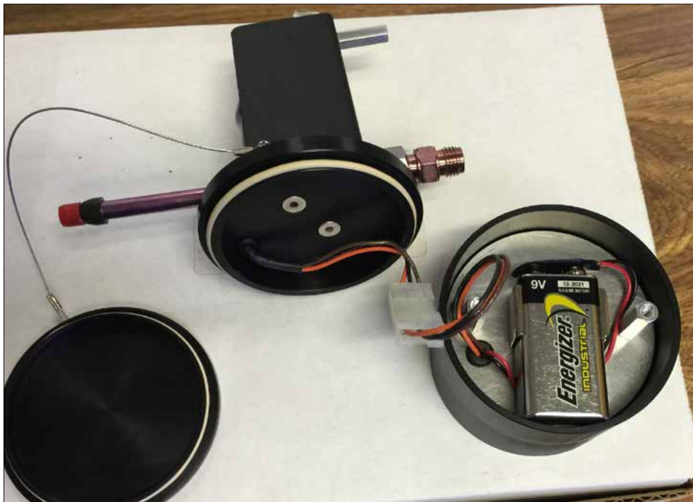
Figure 5.3 - TM1200 Open for Battery Replacement.
