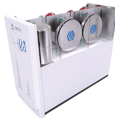
Figure 6 - The two Multi-Capillary Column Trapping Stages are shown above: Stage 1: Trap; Stage 2: Focus. Simple fans are used to cool traps down to 35°C. No complicated electronic cooling makes it easier to operate and maintain by the laboratory chemist.
