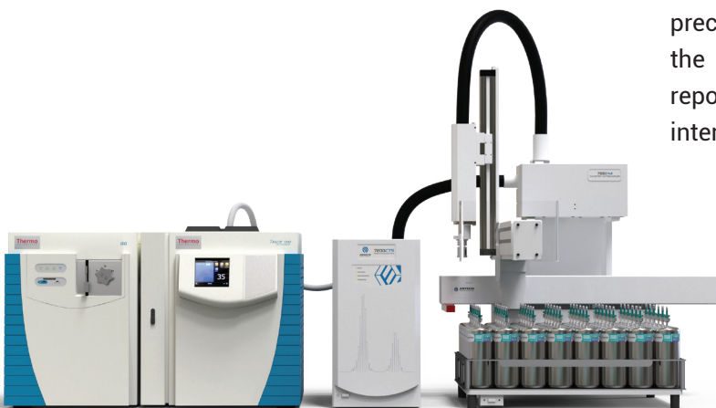
Figure 5 - The 7650 Million Air Autosampler quickly screens six 6L or 3.2L canisters (shown above) for high concentration samples in just over half an hour, therefore 60-80 samples can be screened in an 8 hour shift. One 7200CTS/7650-M can screen enough samples to keep 4-5 other systems safe and productive.
