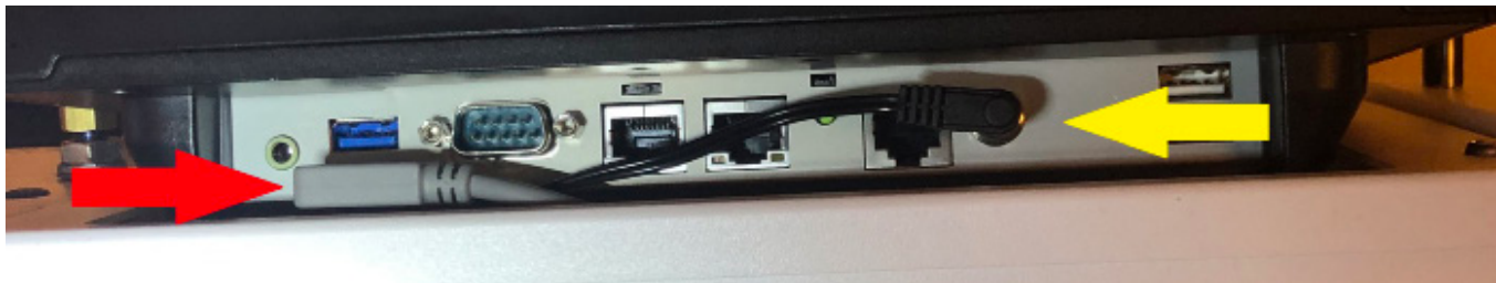
Figure 2.6.5.2. Above. The red arrow shows the internal USB cable connecting to the bottom of the Controller on the front of the 1900. The yellow arrow show the internal computer power cord connecting to the Controller.
