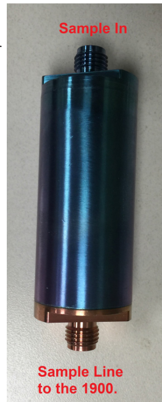
Figure 2.6.10a. Below. Sample Inlet Filter and Orientation.
