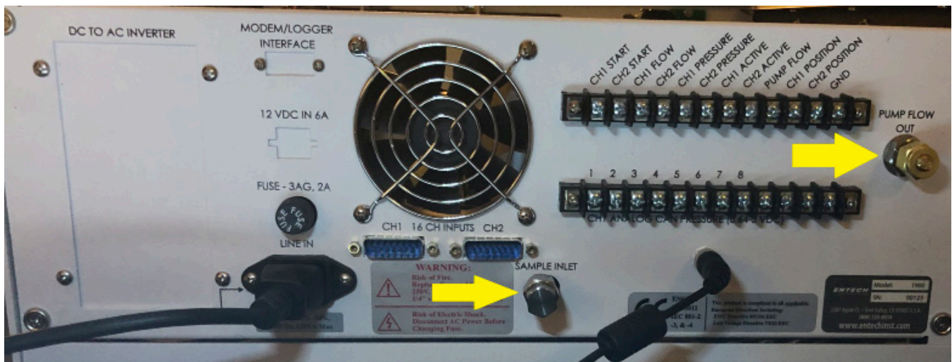
Figure 2.6.7. Above. The yellow arrows point to the Sample Inlet bulkhead and the Pump Flow Out bulkhead.
