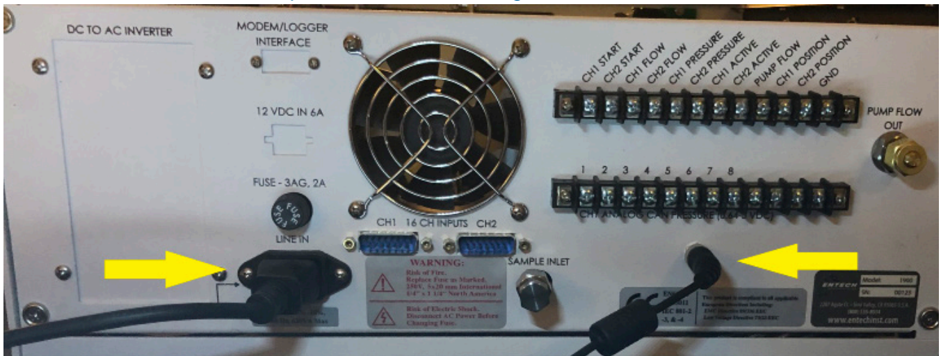
Figure 2.6.5.4. Below. The yellow arrows show the main power cable and the Controller power cable connecting to the rear of the 1900.
