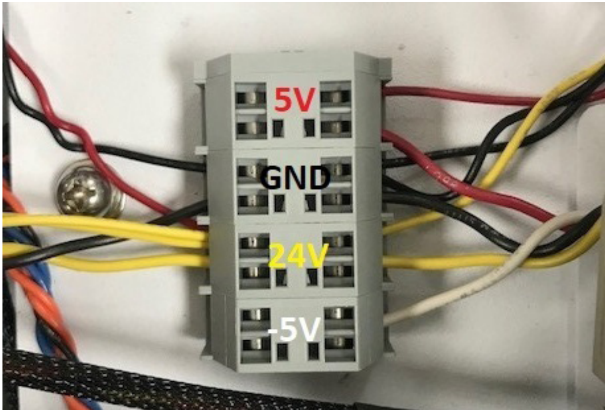
Figure 3.10.3.1. 1900 DC Voltage Distribution Bar.
