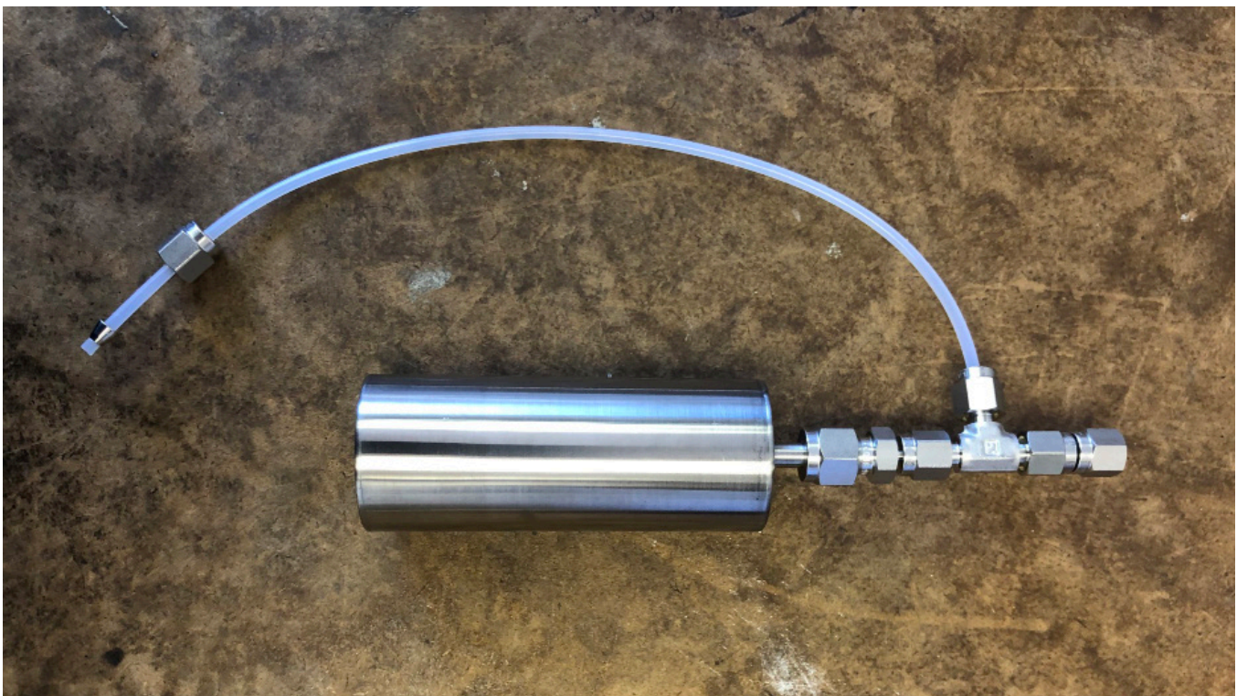
Figure 3.3.2.4. 1900 Calibration Ballast Assembly. The calibration tubing is connected to the ballast/tee assembly.
