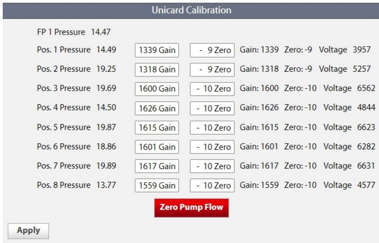
Figure 4-10 Unicard Calibration Screen in the Settings Main Box.
