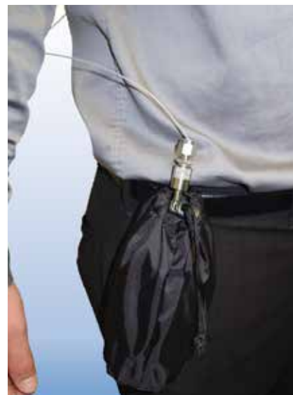
STEL monitoring shown with Silonite™ filtered inlet line sampling directly into a Bottle-Vac™ in pouch attached to belt.
