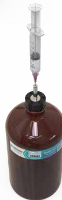
Breath Sampler shown with 1L Bottle-Vac™.
