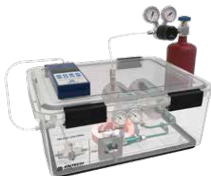
SG-MW-SHR-200-Kit Gas Shroud ensuring >95% soil gas collection
