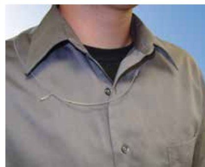
STEL monitoring shown with Silonite™ filtered inlet line sampling directly into a Bottle-Vac™ in pouch attached to belt.
