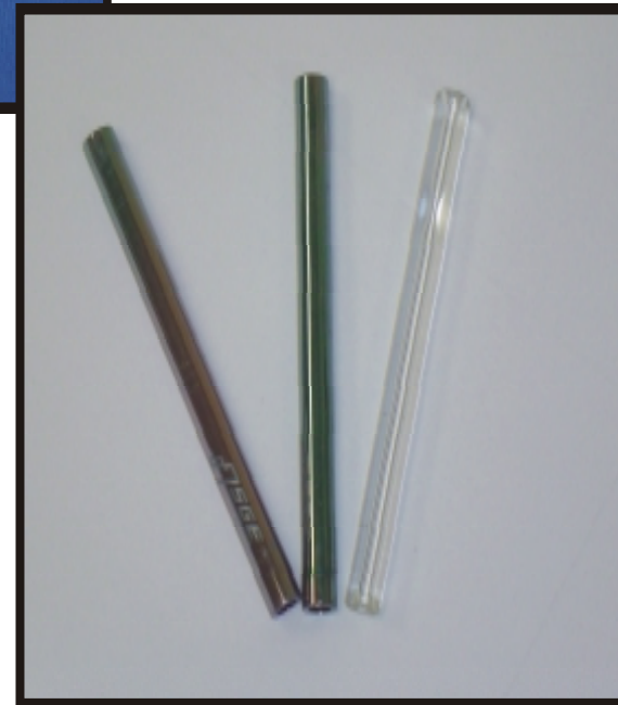
Translucent Silonite Coated Liners next to Uncoated Glass Liner
