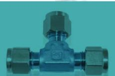
NOTE: Nuts are not coated since they do not come in contact with a sample path. Ferrules are also not coated since Silonite coating would make the surface harder, resulting in variances in sealing characteristics.
