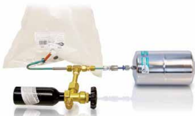
Figure 1 - A \text{CO}_2 Cylinder is attached to the cooling tee during sample collection into a 1.4L MiniCan ™ .
