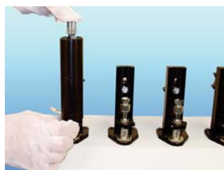
5 Gently snug thumb-wheel on bulkhead fitting and perform pressurized leak check.
